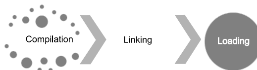
FIGURE 3.1 In C, the compiler converts the source code to the object code. This is followed by links, and finally, memory is allocated to the process.
